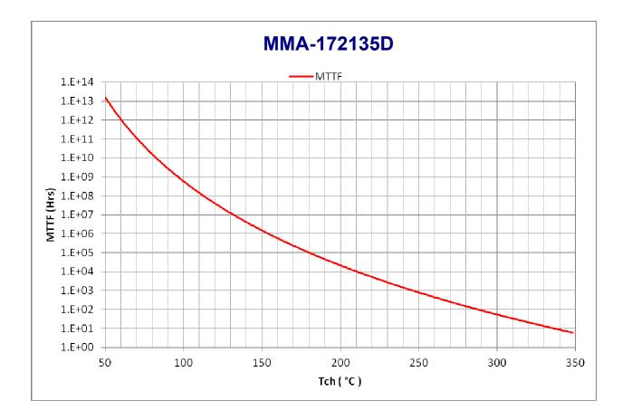
This plot is based on MTTF data provided by wafer foundry and is scaled to the size of this MMIC size.
